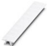
Zack marker strip, can be ordered: Strip, white, labeled according to customer specifications, mounting type: snap into tall marker groove, for terminal block width: 6.2 mm, lettering field size: 6.15 x 10.5 mm, Number of individual labels: 10
