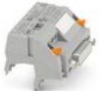
V8 adapter for 8 x PLC-INTERFACE (6.2 mm), controller: PLC system cabling of output cards, connection 1: Screw connection 1x, connection 2: D-SUB socket strip 1x 15-position, connection 3: Plug connection (Can be snapped onto 8x PLC-INTERFACE terminals), number of channels: 8, control logic: plusschaltend
