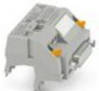
V8 adapter for 8 x PLC-INTERFACE (6.2 mm), controller: PLC system cabling of input cards, connection 1: Screw connection 1x, connection 2: D-SUB socket strip 1x 15-position, connection 3: Plug connection (Can be snapped onto 8x PLC-INTERFACE terminals), number of channels: 8, control logic: plusschaltend
