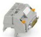
V8 adapter for 8 x PLC-INTERFACE (6.2 mm), controller: PLC system cabling of output cards, connection 1: Screw connection 1x, connection 2: D-SUB pin strip 1x 15-position, connection 3: Plug connection (Can be snapped onto 8x PLC-INTERFACE terminals), number of channels: 8, control logic: plusschaltend
