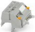
V8 adapter for 8 x PLC-INTERFACE (6.2 mm), controller: PLC system cabling of input cards, connection 1: Screw connection 1x, connection 2: IDC/FLK pin strip 1x 14-position, connection 3: Plug connection (Can be snapped onto 8x PLC-INTERFACE terminals), number of channels: 8, control logic: plusschaltend
