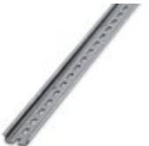
DIN rail perforated, Standard profile, width: 35 mm, height: 7.5 mm, acc. to EN 60715, material: Steel, Galvanized, white passivated, length: 2000 mm, color: silver
