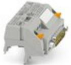
V8 adapter for 8 x PLC-INTERFACE (6.2 mm), controller: PLC system cabling of input cards, connection 1: Screw connection 1x, connection 2: D-SUB pin strip 1x 15-position, connection 3: Plug connection (Can be snapped onto 8x PLC-INTERFACE terminals), number of channels: 8, control logic: plusschaltend
