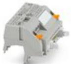
V8 adapter for 8 x PLC-INTERFACE (6.2 mm), controller: PLC system cabling of output cards, connection 1: Screw connection 1x, connection 2: IDC/FLK pin strip 1x 14-position, connection 3: Plug connection (Can be snapped onto 8x PLC-INTERFACE terminals), number of channels: 8, control logic: plusschaltend
