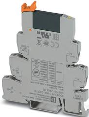
PLC-INTERFACE, consisting of PLC-BSC.../21 basic terminal block with screw connection and plug-in miniature solid-state relay, for mounting on DIN rail NS 35/7,5, 1 N/O contact, input: 24 V DC, output: 3 - 48 V DC/100 mA
